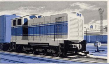
CM6-650-H.P. General Purpose Loc tive-Latest addition to the line of Go Motors Diesel-Electric locomotives, this satile low-cost unit is designed for si where light-axle loading is required. Por by a 6-cylinder 567C 2-cycle engine, three driven axles arranged on a rigidbase with the three axles driven by a carbody-mounted heavy-duty traction r evithrough shafting and gearboxes. Miniweight 36,281 kg.—can be ballasted to i mum of 45,444 kg. Maximum speed 48 All gauges from .914 M. to 1.676 M.
